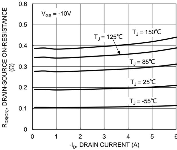
Figure 17. Typical On-Resistance vs. Drain Current and Temperature
